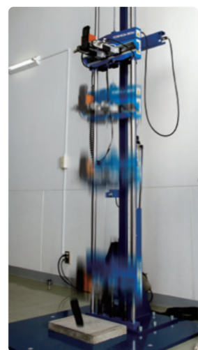
Drop durability test
