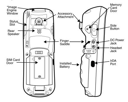
\*Pull the plastic tab to remove the plastic film cover over the image engine window before activating the image engine.
